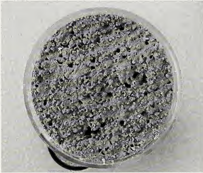
Figure 20. Surface view of the sediment core that was used in the Haines apparatus (Haines, 1930). Two categories of burrow opening are clearly visible. The large ones are the openings of the U-shaped burrows of adult mud shrimp, Corophium volutator . The smaller ones are the openings of similar U-shaped burrows constructed by small immature Corophium volutator . These field cores when brought to the lab are completely drained of pore water.
